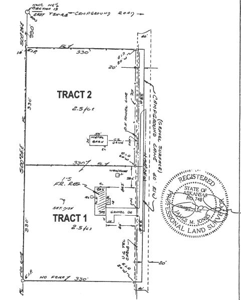
CERTIFICATION: THIS IS TO CERTIFY THIS PLAT AS BEING THE RESULTS OF A FIELD SURVEY MADE BY ME ON 5/19/94 BASED ON EXISTING MONUMENTS AND PLATS FOUND IN AND OF THE AREA AND IS TRUE AND CORRECT TO THE BEST OF MY KNOWLEDGE, IMPROVEMENTS ARE AS SHOWN. THIS PROPERTY DOES NOT LIE WITHIN A DESIGNATED FLOOD ZONE AS PER FLOOD HAZARD BOUNDARY MAP, WHITE COUNTY, AR. COMMUNITY PANEL NO 050467 0013 A AND DOES NOT LIE WITHIN ANY DESIGNATED ZONE.
